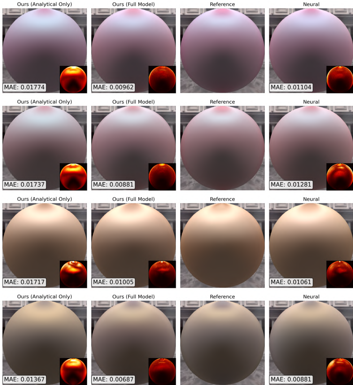
Figure 12: Results on the UTIA dataset. From top to bottom: m071_fabric106, m072_fabric107, m074_fabric111 and m075_fabric112. The MLP size is 32 \times 3 , and the latent vector is set to l = 4 for our hybrid model and l = 12 for the Neural model.
